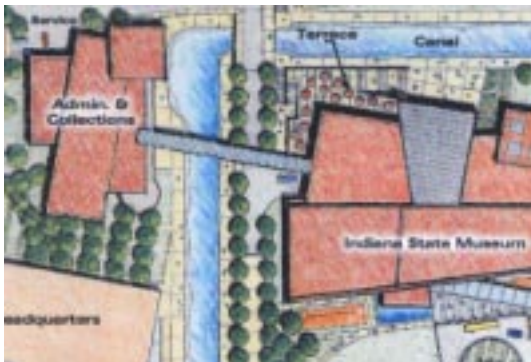
Above Left: A 200 ft. bore under a canal and roadway was needed to connect the Indiana State Museum with the new Administration Building. Above Right: Prime Conduit Bore-Gard has a 65 degree bend radius making it flexible enough to be pulled around a building.
